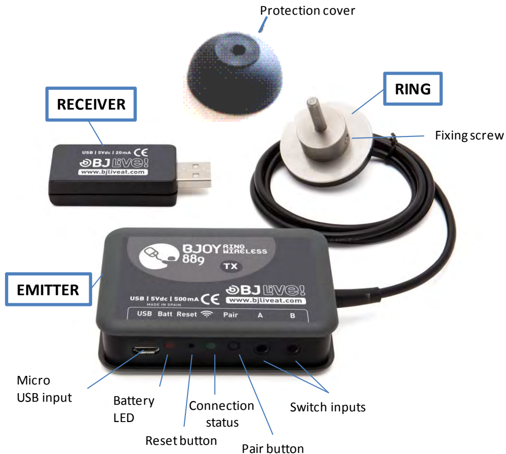
Fig. 1: Parts of the BJOY Ring wireless
